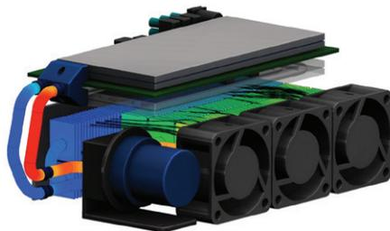
Liquid cooled autonomous vehicle sensor fusion box.
